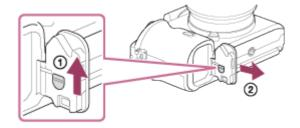
• You can attach the removed battery cover to the vertical grip so that you do not lose it.
