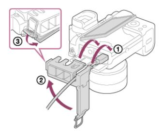
• Make sure the connector cover is outside the cable protector when you attach the cable protector.
