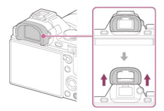
Adjust the diopter scale to your eyesight until the display appears clearly in the viewfinder. If it is difficult to turn the diopter-adjustment dial, remove the eyepiece cup and then adjust the dial.
