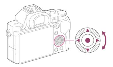
You can select setting items by turning or pressing the top/bottom/right/left side of the control wheel. Your selection is determined when you press on the center of the control wheel.
