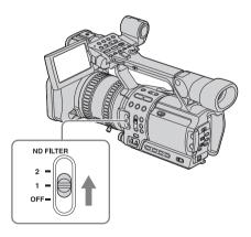
If [ND1] or [ND2] flashes in the standby mode, set the ND FILTER switch to the respective position.
