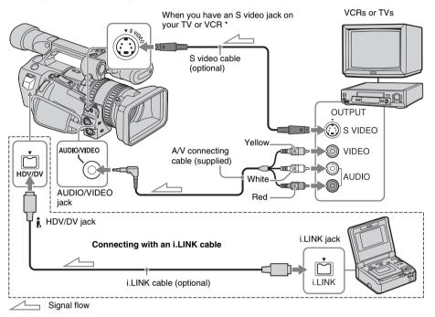
\* When there is an S video jack on the device to be connected, connect an S video cable (optional) to that jack instead of using the yellow video plug of the A/V connecting cable (supplied). This connection produces higher quality DVCAM (DV) format pictures. The audio will not be output if you connect with the S video cable alone.
