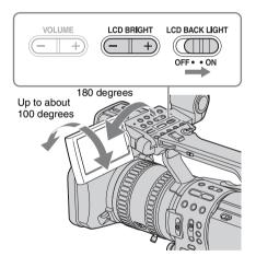
Open the LCD panel 180 degrees, then rotate it to the desired position.
