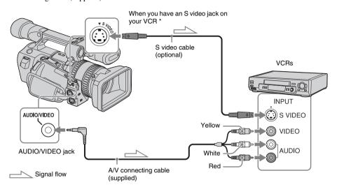
\* When there is an S video jack on the device to be connected, connect an S video cable (optional) to that jack instead of using the yellow video plug of the A/V connecting cable (supplied). This connection produces higher quality DVCAM (DV) format pictures. The audio will not be output if you connect with the S video cable alone.
