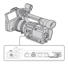
**1** During recording or in the standby mode, set the AUTO LOCK switch to the center position to release the auto lock mode.
