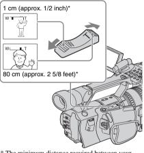
\* The minimum distance required between your camcorder and the subject to get a sharp focus with that side of the lever.
