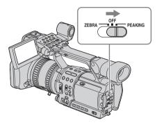
During recording or in standby mode, set the ZEBRA/PEAKING switch to PEAKING.
