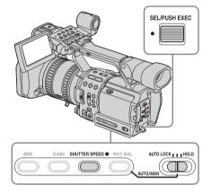
**1** During recording or in the standby mode, set the AUTO LOCK switch to the center position to release the auto lock mode.
